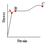
In the region from 0 to A, the curve is linear. The strain is directly proportional to the stress. Beyond the point A, known as the proportional limit, the relation between stress and strain is not linear.
