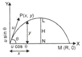
Suppose a body is projected with velocity u at an angle  $\theta$  with the horizontal, P(x,y) is any point on its trajectory at time t. Horizontal component of velocity is unaffected by gravity, but the vertical component ( $u \sin \theta$ ) changes due to gravity.
